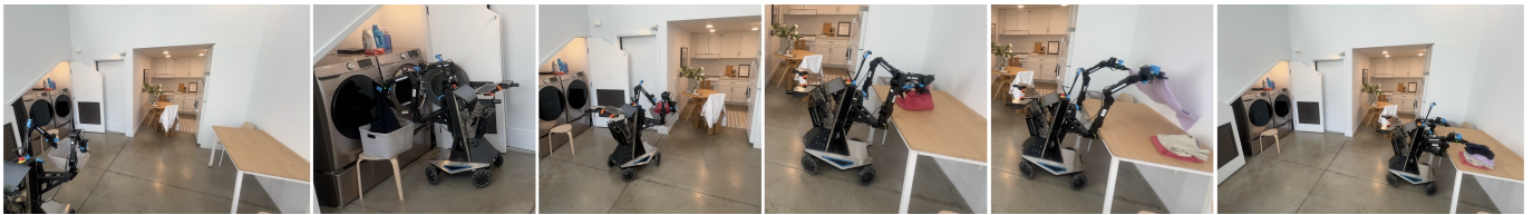
Fig. 2: \pi_0 controls a mobile manipulator to fold laundry. Our model is pre-trained on diverse data from 7 distinct robot configurations and 68 tasks, and can then be used in zero-shot or fine-tuned to complex downstream tasks, as in the case of this laundry folding policy, which fetches laundry from a dryer, packs it into a hamper, brings the hamper to a folding table, and then folds each article of clothing.
