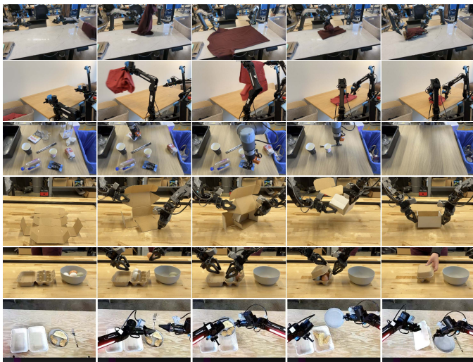
Fig. 12: We evaluate a range of complex and temporally extended tasks. This includes: folding laundry from a bin with a stationary (a) or mobile (b) robot, bussing a real lunch table (c), assembling a box (d), packing eggs into a carton (e), and packing food into a to-go box (f). These tasks require combining dozens of individual behaviors, such as grasping, stacking, folding, and flattening, generalization to a huge variety of object configurations, and complex physical properties, such as deformable objects or flexible cardboard.
